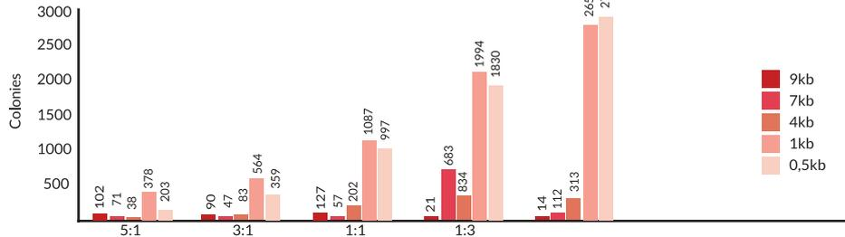
Efficiency of cloning pSpark® I inserts of different sizes using different vector: insert ratios. Inserts were used 0.5 kb, 1kb, 4kb, 7kb and 9kb in the ratios indicated below. Competent cells were  $2 \times 10^7$  cfu/ $\mu$ g DNA. Background was always below 1%.
